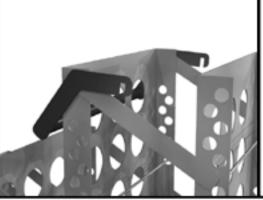
Rotate the locking arm so that it clears the structure.
