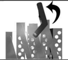
Disengage the locking arm/handle by pushing the handle towards the back of the system.
