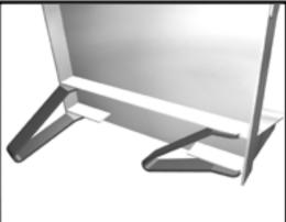
Locate the feet on the back of the unit. Fold the feet out.
