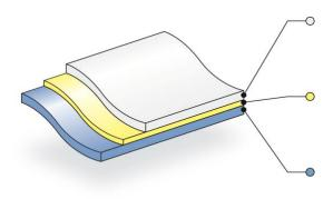
Facestock: 1.5 mil clear film with outstanding outdoor durability. Offering excellent dimensional stability combined with good solvent, elevated temperature, and UV resistance.
