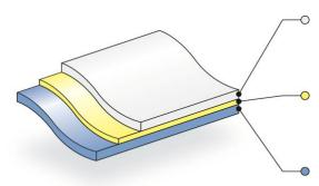
**Facestock:** 2 mil optically clear topcoated polyester features a minimum of 80% recycled polyester content. It offers excellent clarity and dimensional stability combined with good high temperature and humidity resistance. The optically clear polyester provides high resolution imaging with excellent
