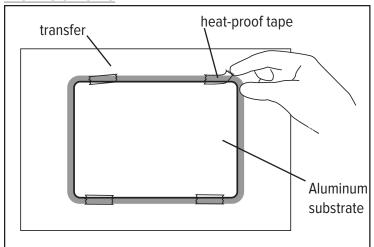
**ALUMINUM:** Peel film, and clean panel with all-purpose cleaner, a cloth, and compressed air. Align panel with transfer and place four pieces of tape along the long sides as shown. Larger panels may require more tape. Press face up. After pressing, remove transfer and allow to cool.
