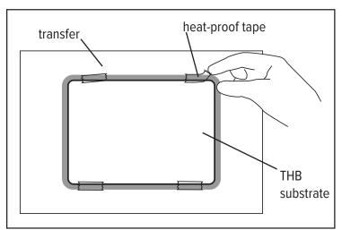
**THB:** Peel film and clean panel with all-purpose cleaner, a cloth, and compressed air. Align panel with transfer and place four pieces of tape along the long sides as shown. Larger panels may require more tape. Press face up. After pressing, remove transfer and allow to cool.
