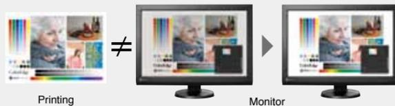
Adjust the screen color tone (whiteness) until it approximates the appearance of the printed output. If the screen output seems blue, move the pointer away from the blue spectrum and toward the red end of the spectrum to remove excess blue.
