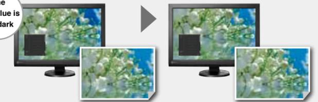
If the light blue on the monitor is too dark when compared with the printed output, move the Hue B (Blue) cursor to the left.
