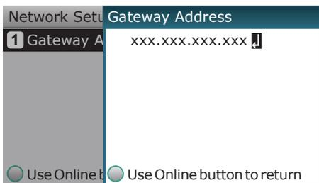
**14** Press the [ON LINE] button to complete the network setup.
