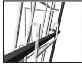
Place the bottom hook of the literature stringer over the bottom literature stringer into the holes in rail.
