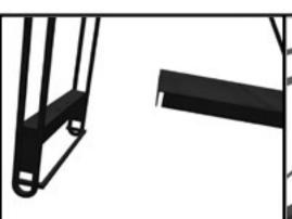
Place the metal plate on the bar at Place the top hook of the literature the bottom of the base of the unit. stringer over the top rail. Make sure that it fits in the groove.
