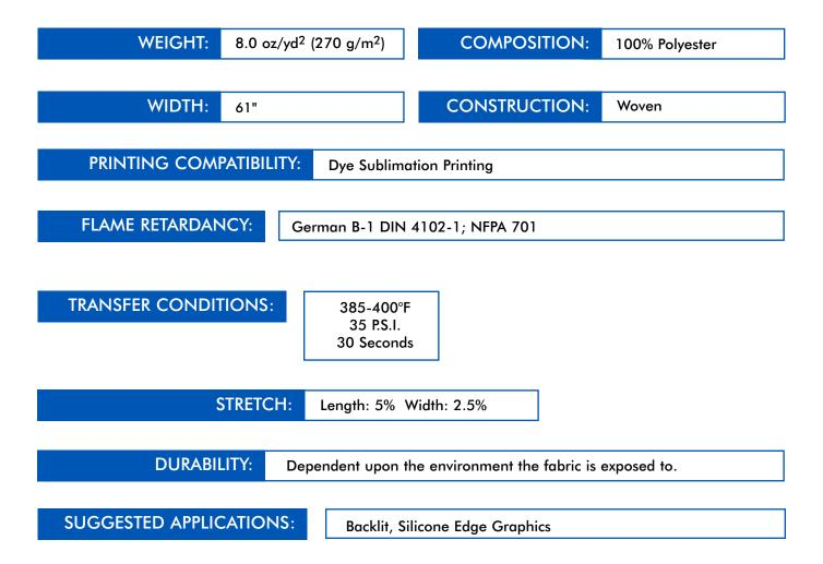
The above recommendations are a result of laboratory testing. We recommend additional testing in the manufacturing facility prior to printing. Data are averages achieved for actual production runs. Product safety evaluations may not have been completed for the intended use. Samples of this product should be used for concept evaluations only.
