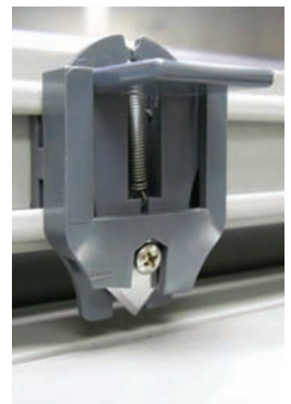
Cross cutter permits simple cutoff as the laminated material exits the rear
