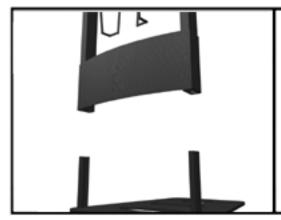
Insert the bottom section of the literature rack onto the foot. Make sure the pockets are facing away from the foot.
