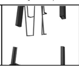
Find the top section of the rack which Place the top section of the literature rack onto the bottom section. Make sure the pockets are facing away from the foot.
