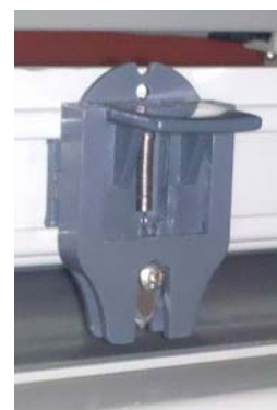
Cross cutter permits simple cutoff as the laminated material exits the rear of the machine
