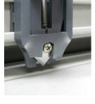
Cross cutter permits simple cutoff as the laminated material exits the rear
